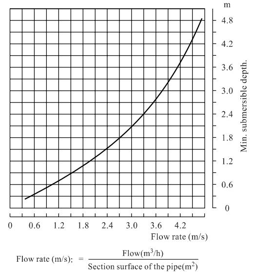
Suggested suction pipe submersible depth VS flow rate
